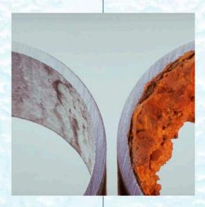
**Soft water** is aggressive on metals and causes corrosion. Consequently the tap water turns brown. Leaks and burst pipes may be the result.
